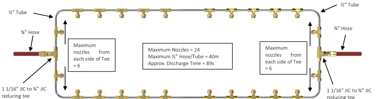
Figure 9 Maximum Distribution Limits for a 2 x C106 configuration
