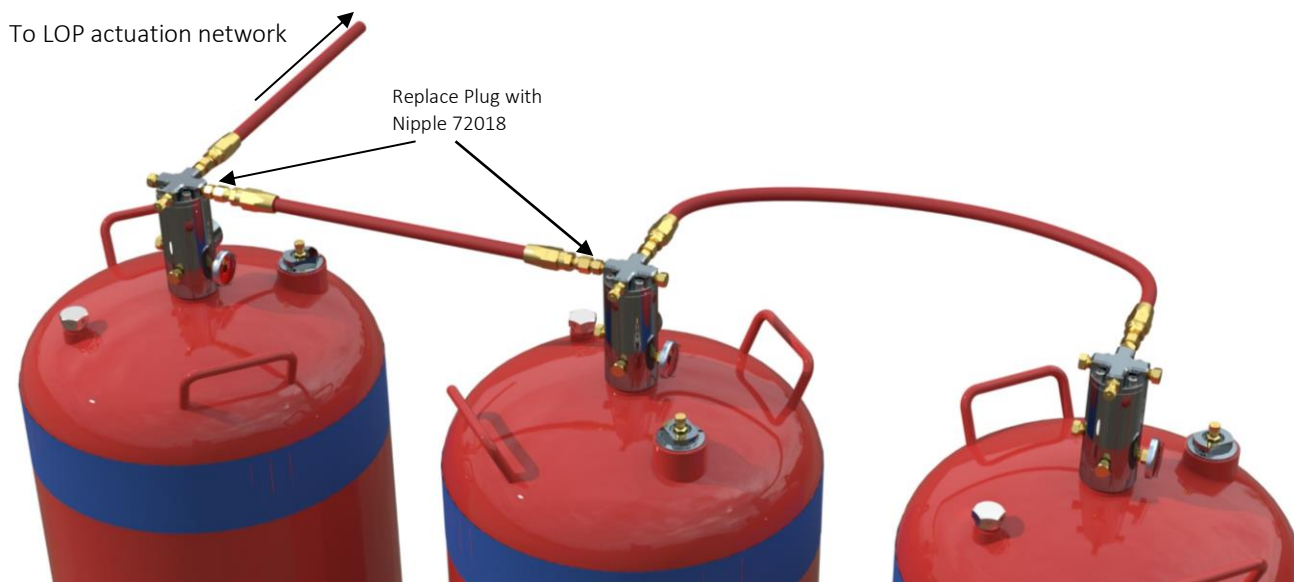
Figure 33 - LOP multiple cylinder actuation arrangement
