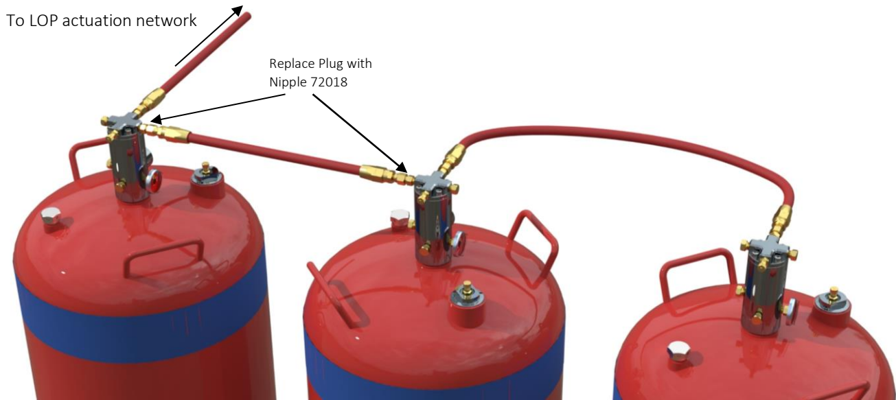
Figure 33 - LOP multiple cylinder actuation arrangement
