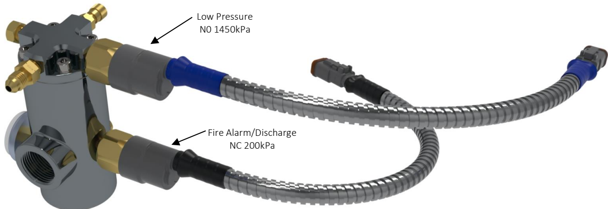
Figure 33 –Pressure Switch mounting location on cylinder valve
